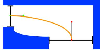
Figure 4: Bézier curve (in orange) through doors (green and red dots) are Bézier way-point for each door and blue area are walls).
