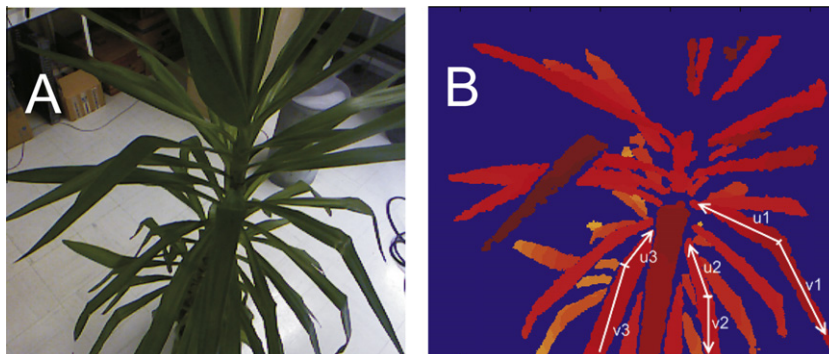
Fig. 4. (A) RGB image of the considered plant for leaf curvature measurement. (B) Depth image of the plant of (A). White arrows indicate the pairs of vectors (\vec{u}, \vec{v}) forming the two planes of the leaves. Angles between these vectors are given in Table 1.
