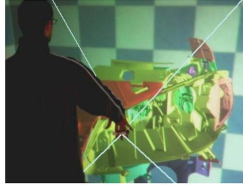
Fig. 5: Picture of a user accessing a hidden part of the virtual mock-up with the SPIDAR.
