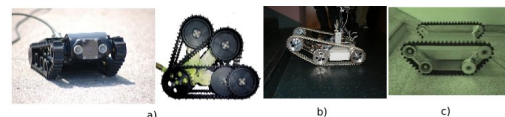
Fig. 3. a) : Micro VGTV (manufacturer: Inuktun Ltd) b) : B2P2 prototype c) : VGSTV mechanism
