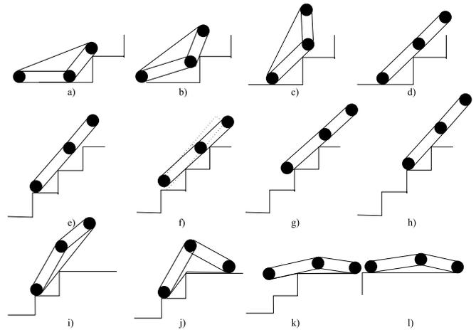
Fig. 10. Clearing of a staircase
