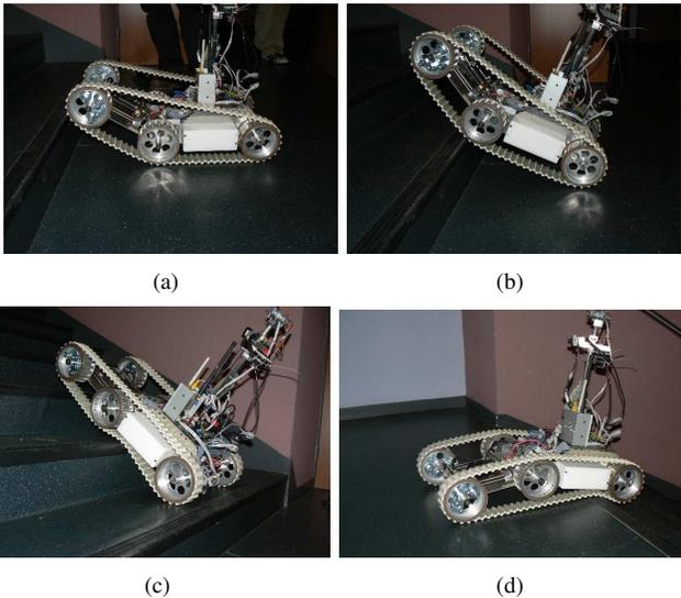
Fig. 9. Clearing of a staircase : pictures
