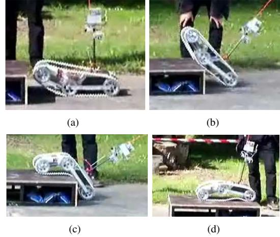
Fig. 8. The clearing of the curb
