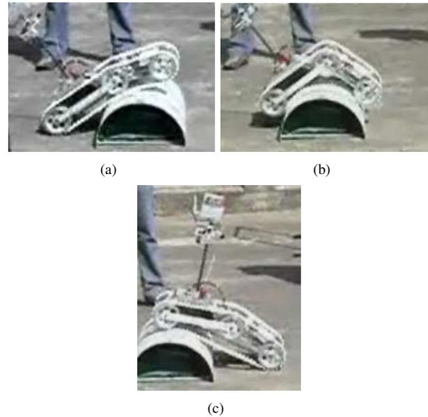
Fig. 11. Clearing of a bumper : pictures
