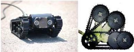
(a) Micro VGTV (Variable Geometry Tracked Vehicle manufacturer: Inuktun Ltd). Photo courtesy of Inuktun Services Ltd.
