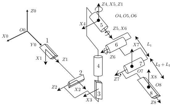
Fig. 6. B2P2's geometric model. The robot is decomposed into three segments. The first is situated between joints 6 and 7, the second starts at the joint 7 and the third at the joint 8.  $L_1$ ,  $L_2$  and  $L_3$  represent respectively the length of the segments 1, 2 and 3.
