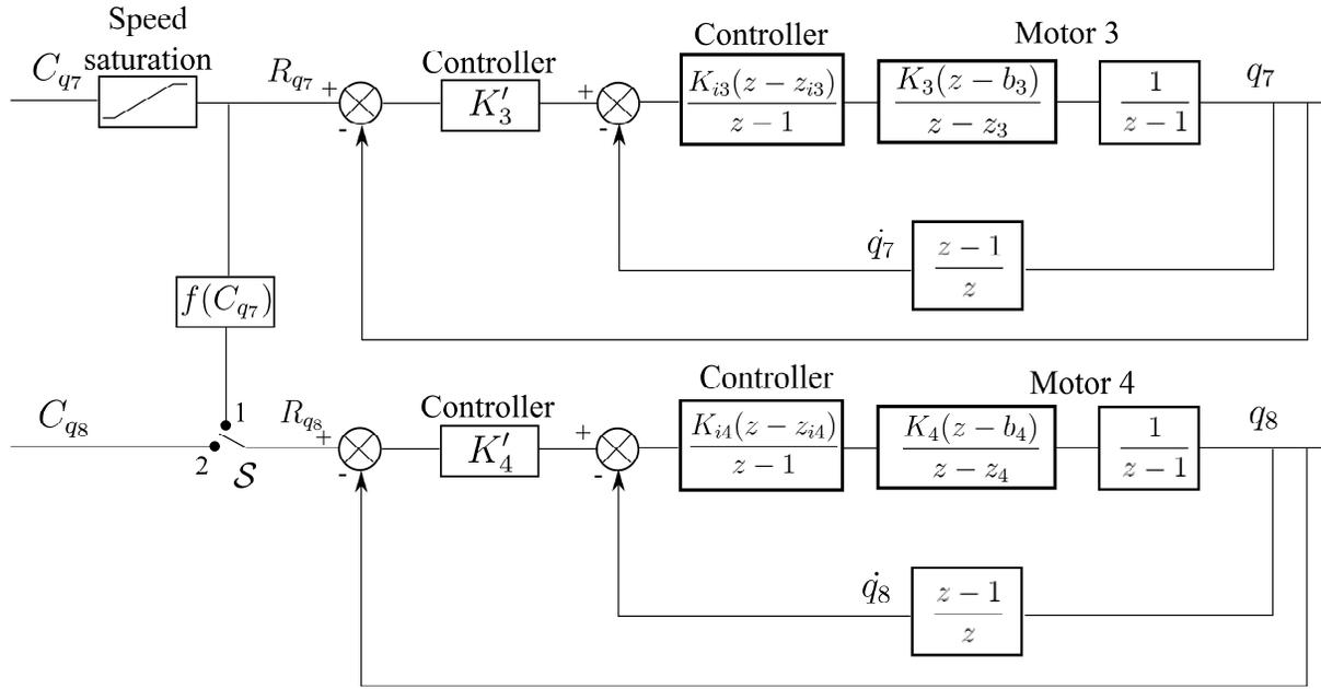
Fig. 7. Elevation/translation control system
