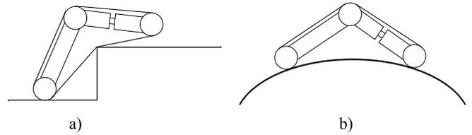
Fig. 5. Different configuration of B2P2 on obstacles. In a), the caterpillars are tense, and in b), they are not to increase the contact surface. Note that even if the system is turn on, the caterpillars are not hardly tense ; it allows soft mass transfer and clearing
