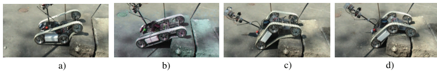
Fig. 3. B2P2 : clearing of a curb
