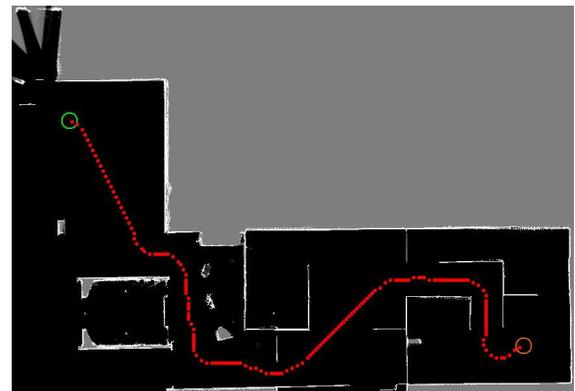
Fig. 8. Example of a planned trajectory keeping away from obstacles
