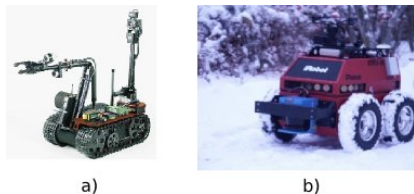
Figure 1: a) : Talon-Hazmat robot (Manufacturer : Foster-Miller) b) : ATRV-Jr robot. Photo Courtesy of AASS, Örebro University
