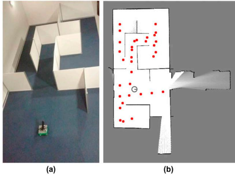
Figure 7. (a) represents the experimental environment. (b) represents the considered map obtained by performing a SLAM algorithm. White cells represent free spaces in the environment, black cells represent obstacles and grey cells represent unexplored spaces. Note that the grey circle in (b) corresponds to the pose of the robot depicted in (a) and the filled points correspond to the 33 performed global localizations.
