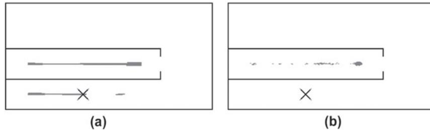
Figure 14. (a) represents the IAL results and (b) the MCL results (the grey shapes). The crosses correspond to the expected result. Note that the best particle of the MCL algorithm is the one depicted in (b). In those conditions MCL fails to estimate the robot's pose while the IAL algorithm results still contain the solution.
