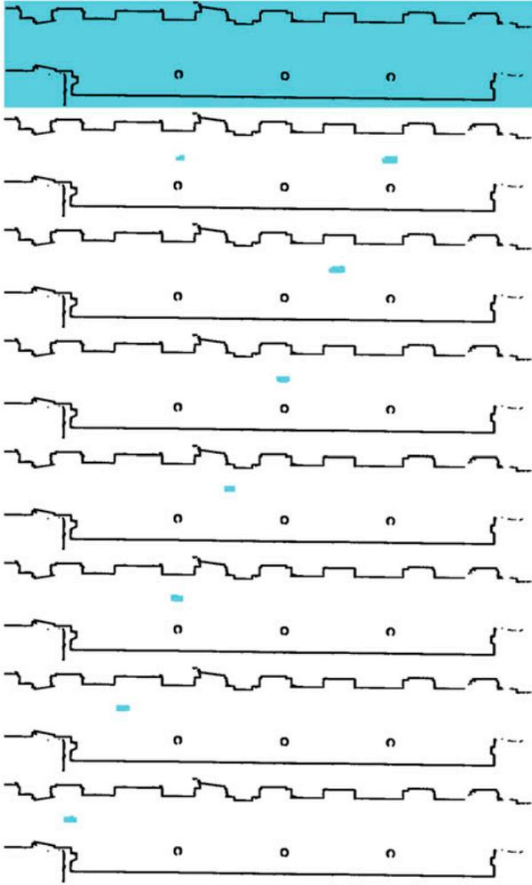
Figure 11. The initial data of the localization problem (first picture), and the seven iterations processed by the IAL algorithm (the first picture correspond to  $k = 0$  and the last one to  $k = 7$ ). It can be noticed that the robot does not move between the times  $k = 0$  and  $k = 1$ .
