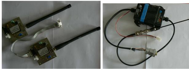
(a) Radiometrix 152.575 MHz transmitter (b) Adeunis 868 MHz RF Modem
