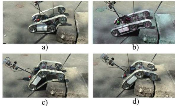
**Fig. 6.** B2P2 : clearing of a curb
