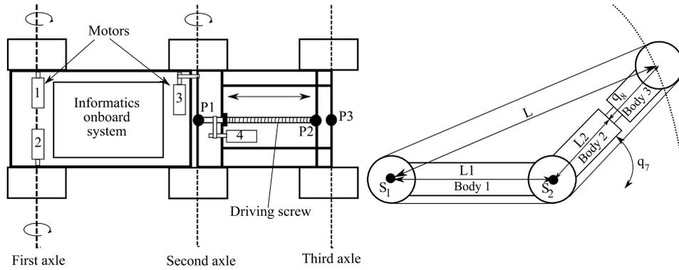
**Fig. 4.** Overview of the B2P2 mechanical structure.
