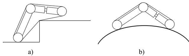
**Fig. 5.** Different configuration of B2P2 on obstacles. In a), the caterpillars are tense, and in b), they are not to increase the contact surface. Note that even if the system is turn on, the caterpillars are not hardly tense ; it allows soft mass transfer and clearing
