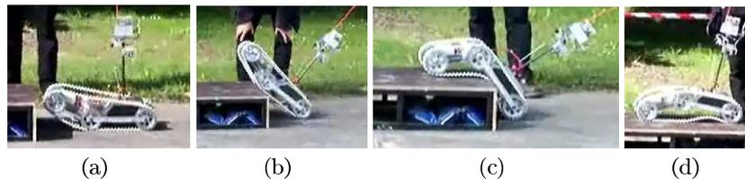
**Fig. 10.** The clearing of the curb
